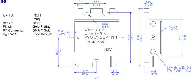
!!Warning: Only use 3/16" long #2-56 screws to mount the SMA connectors. Longer screw may damage the internal components.
