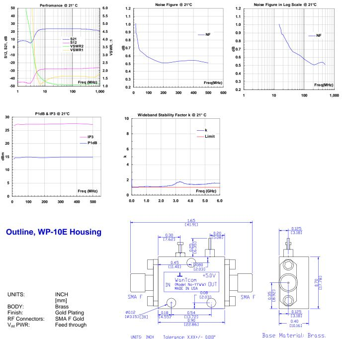
Base Material: Brass. Finish: Gold Plating. RF I/D: SMA Female
