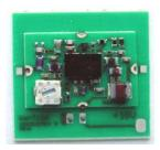
Fig. 3 Assembled preamp
