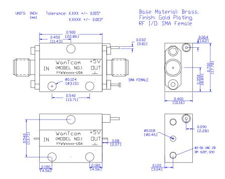
For the pin type input and output application, remove the input and output SMA connectors.
